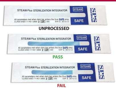
**STEAMPlus™ Class 5 Integrators** are used with steam sterilization cycles to provide a definitive **pass or fail result** – allowing for the release of all non-implant loads before the results of the spore test are received.
